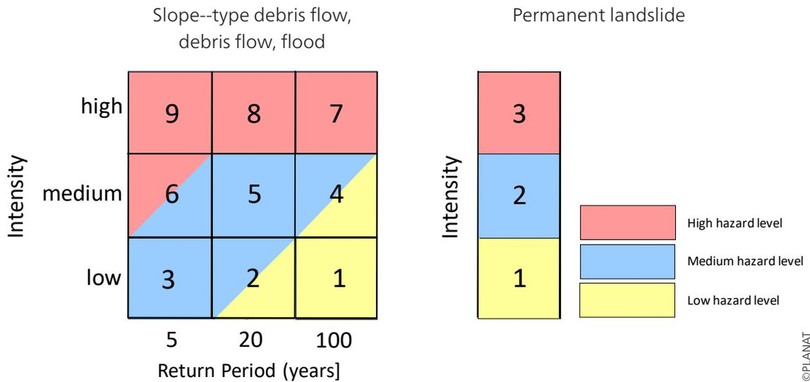
Illustration 2: Hazard level diagram for slope-type mud flows, debris flows and floods (left). No return periods are defined for the „permanent landslide“ process; only the intensity criterion defines the hazard level (diagram to the right).
