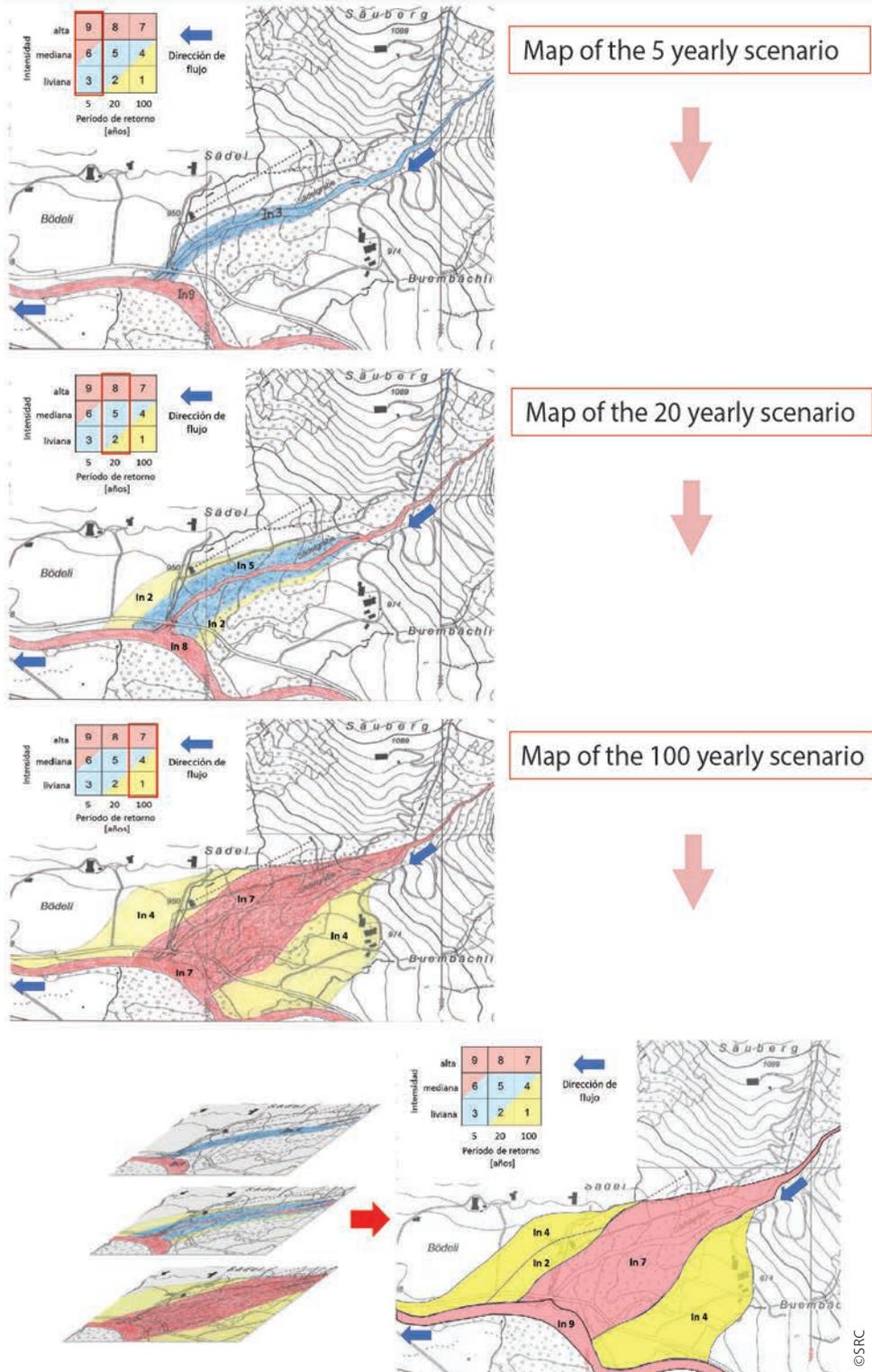
Illustration 3: Mapping of flood scenarios for different return periods and compilation of a flood hazard map (map below to the right). Blue arrow shows the flow direction of the torrent.
