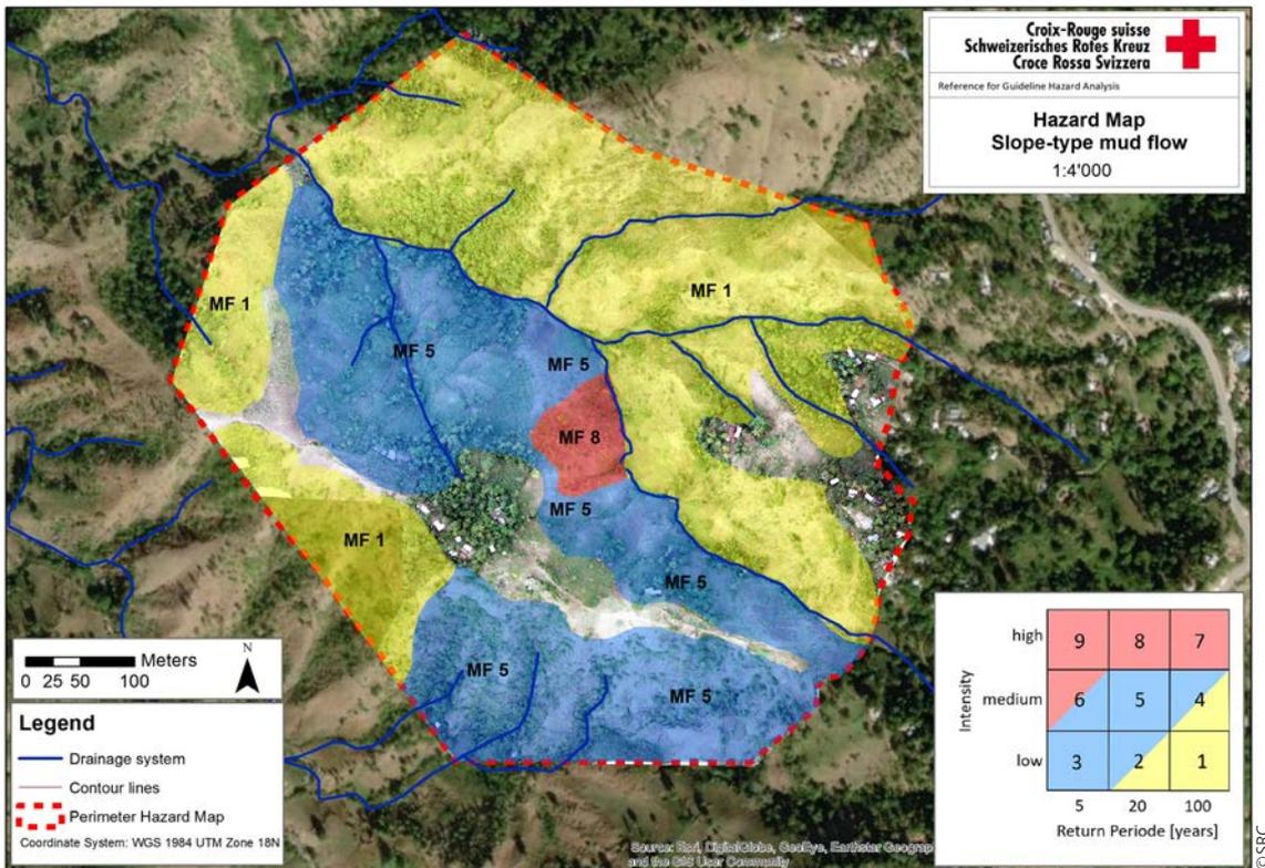
Illustration 5: Slope-type mud flow hazard map in Léogâne, Haiti. The indices are marked with the acronym „MF“ for „MudFlows“.
